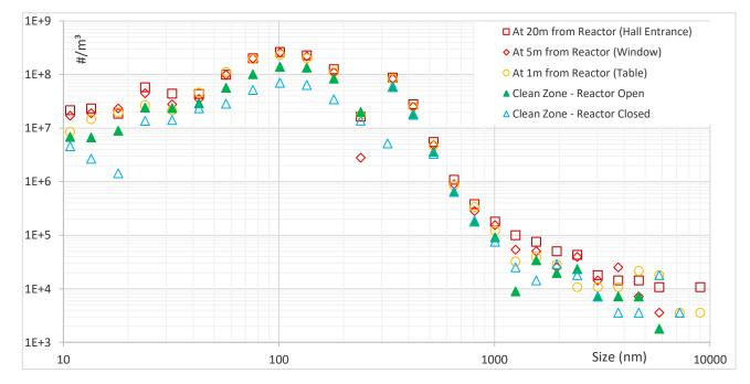
$\rightarrow$  An increase of particle counts from 4,09 to 7,22.10<sup>8</sup> #/m<sup>3</sup> is observed in the immediate surrounding, when the reactor is opened.
