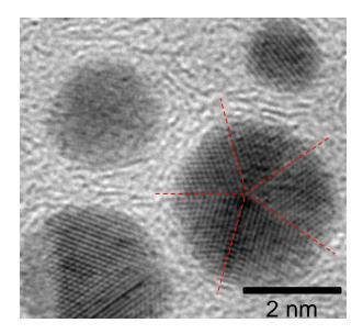
Single Ag nanoparticles (TEM image) with lattice parameter a=237 pm in (110) orientation corresponding to that of 99.999% pure silver <sup>[1]</sup>
