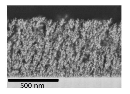
$\rightarrow$  NPs aggregates are produced in vacuum, carrying electric charges and tend to (weakly) adhere to surfaces thanks to electrostatic forces. As the system is put back to atmospheric pressure, they may be expected to mostly remain fixated on solid surfaces.
