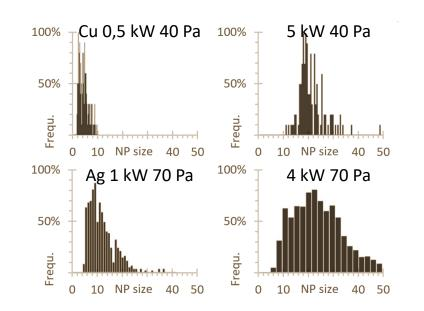
→ Clusters and NPs are generated with sizes ranging from a few nm to 50nm.
