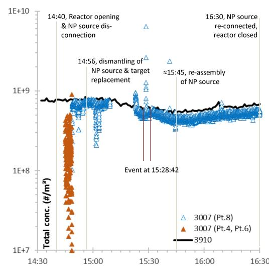
In typical maintenance operation, operators disconnected NP gas aggregation source, dismounted it and changed targets on the workbench. Particle count was acquired at Window (Pt.5, 3.75 m away, solid line) and from the handheld 3007 moved in and out laminar flow cabinet (Pt.4 and 6,  $\blacktriangle$ ) and workbench (Pt. 8,  $\triangle$ )
