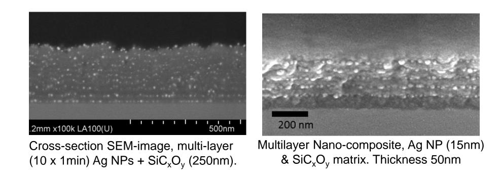
$\rightarrow$  NPs are generally included in a solid matrix attached to substrate. Nanocomposites are obtained by alternating NPs and filler material depositions.
