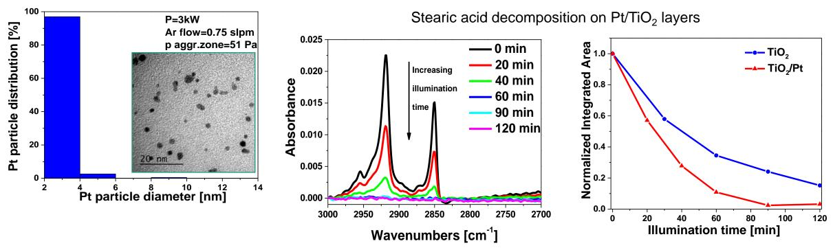
Pt NPs with narrow size and size distribution can be deposited by Gas Flow Sputtering
