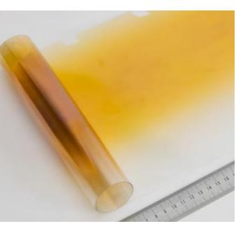
Absorption wavelength can be adjusted by tuning NPs size and NP distribution (Increase of particle size: redshift of the SPR peak) Plasmonic coating on flexible substrate (200x1200mm), Ag NP in isoprene matrix deposited during continuous rotation of the sample holder
