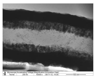
Complete intermixture of NPs in the matrix by fast sample holder rotation (TEM image)
