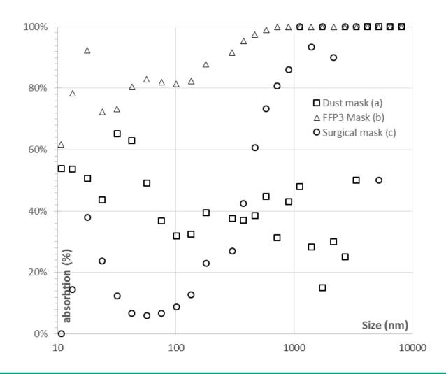
$\rightarrow$  FFP3-rated masks appear to be the best recommendation for the operator protection with permeability of 20% is observed in the 10...100nm range
