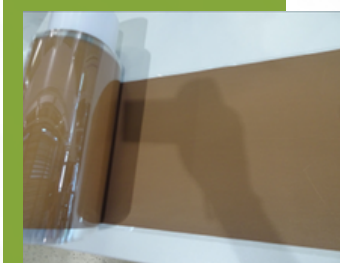
Functionalized PA membrane with Au-coating
