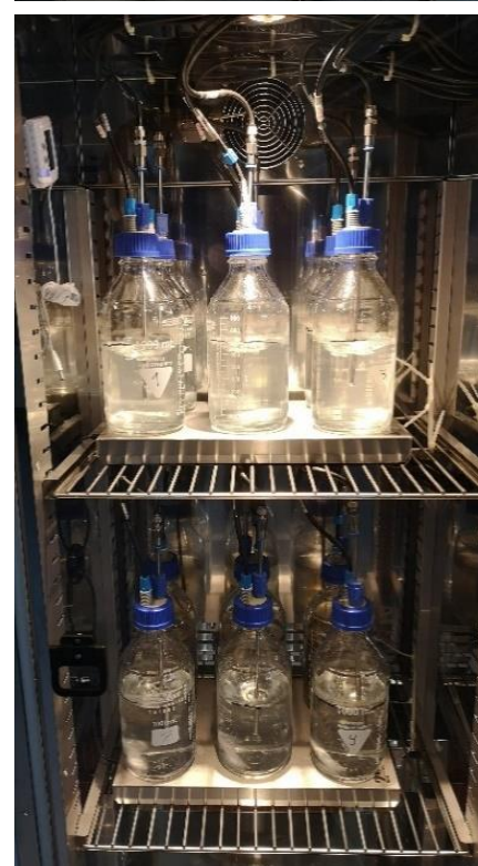
Figure 3: Respirometer allows the monitoring of the release of CO 2 over time in the compost or the marine environment
