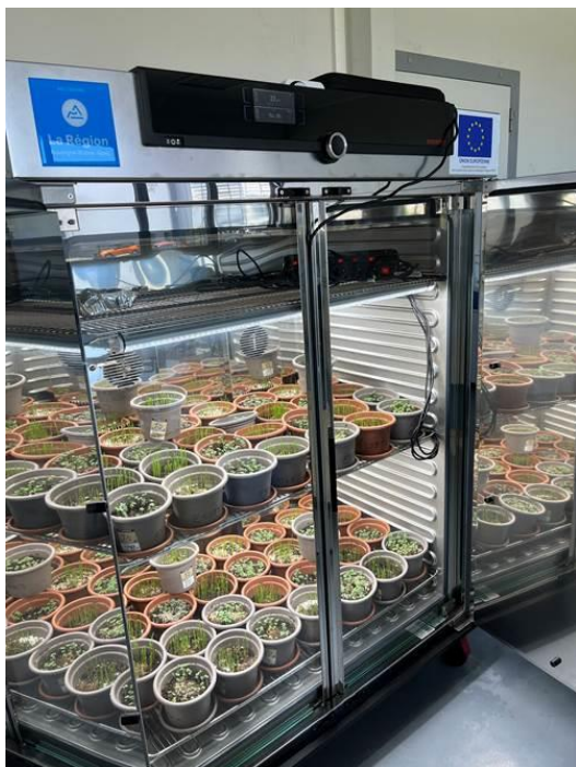
Figure 7: The climatic chamber allows the incubation of plants with controlled humidity, temperature and light.
