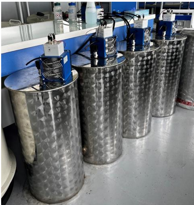
Figure 5: Decay vessel used for pilot scale standard. Tracks home and industrial composting
