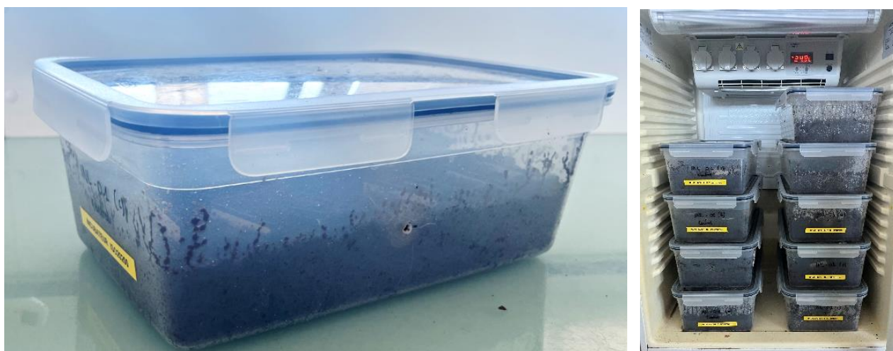
Figure 4: Incubator for the study of disintegration on a laboratory scale
