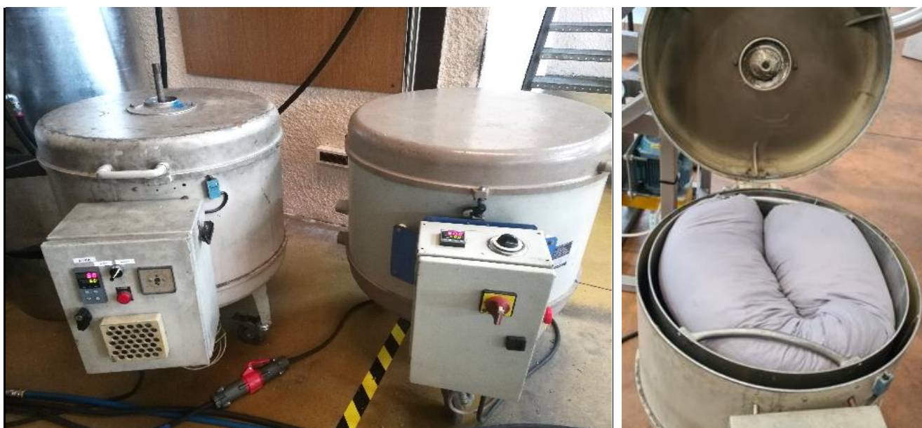
Figure 9: Industrial oven (left: outside view, right: with fabric bags)
