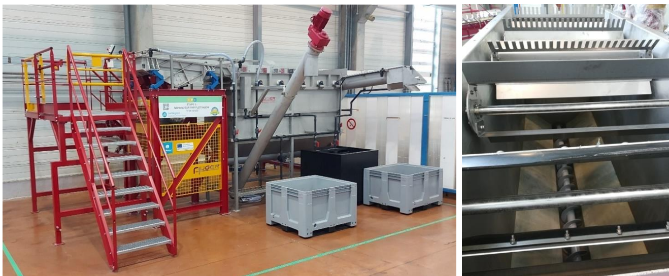
Figure 8: Dynamic flotation bath (left: outside view, right: inside view)
