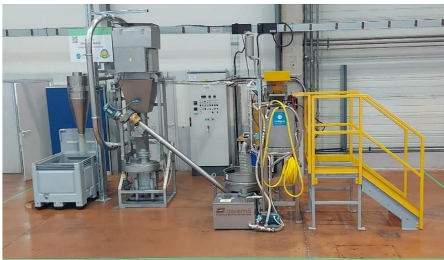
Figure 7: Washing module (left: dryer & cyclone, right: washing tank)
