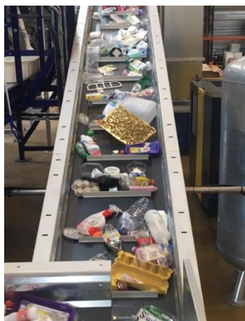
Figure 18: Loaded conveyor belts with mixed stream
