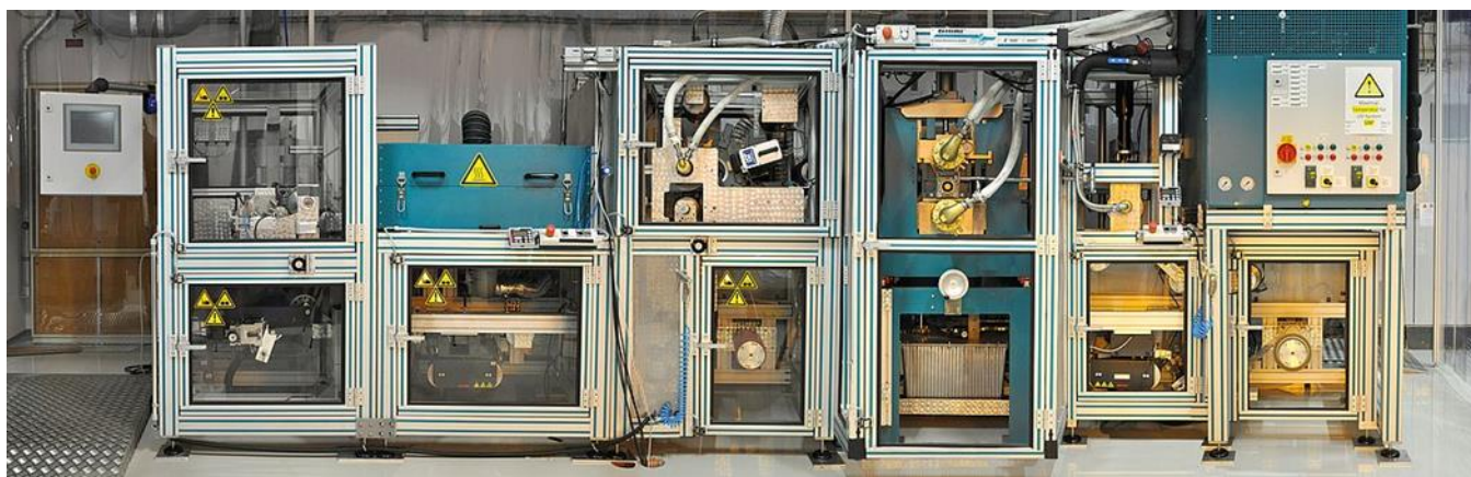
Figure 12 Roll-to-roll machine for UV nanoimprint lithography at JOA
