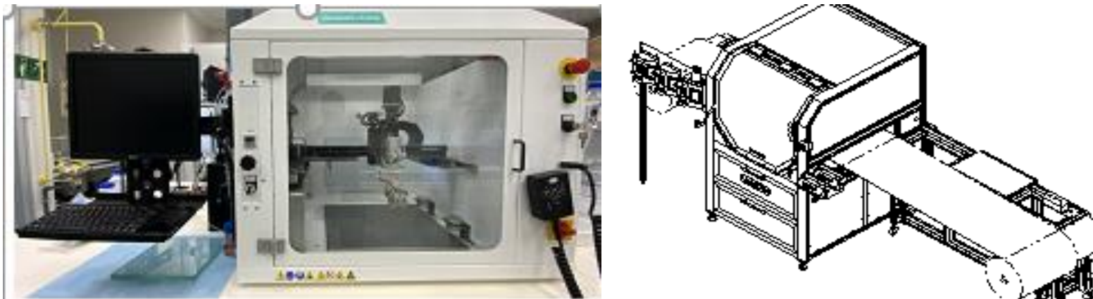
Figure 10: Picture and scheme of the ultrasonic spray coating machine
