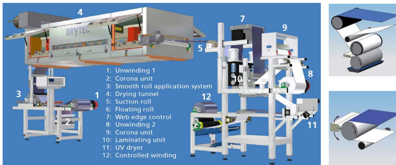
Figure 8: (Left) Scheme of the roll-to-roll wet chemical coating and lamination pilot line at Fraunhofer IVV. (Right) Scheme of reverse gravure and slot-die coating technique
