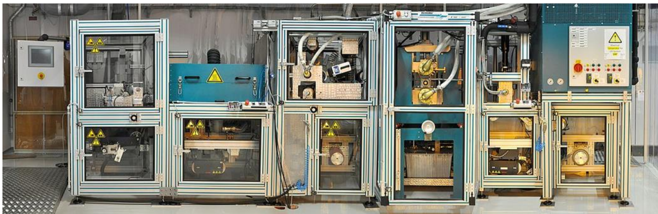
Figure 12 Roll-to-roll machine for UV nanoimprint lithography at JOA
