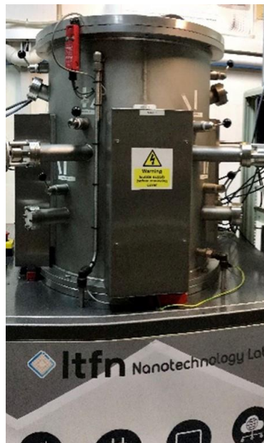
Figure 6: Picture and scheme of the sheet-to-sheet magnetron sputter system
