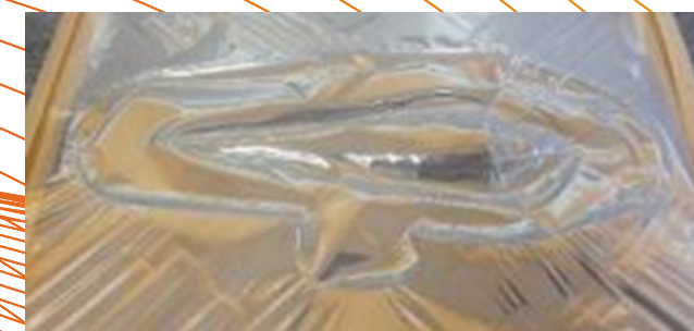
First thermoforming trials at IPC and CRF of a 100 \mu\text{m} thickness foil
