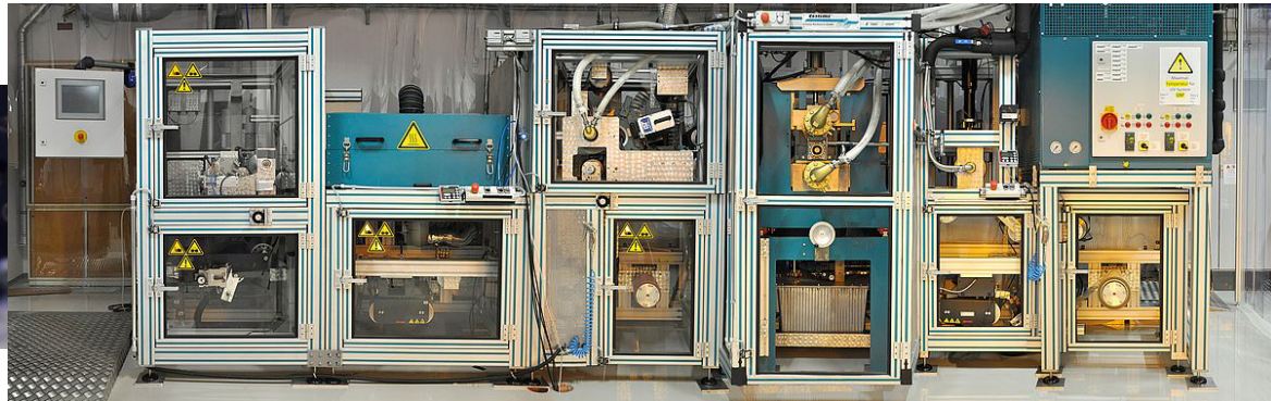
Roll-to-roll machine for UV nanoimprint lithography at JOANNEUM RESEARCH
