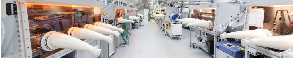
Panoramic view into the cleanroom at Fraunhofer IAP with sheet-to-sheet pilot line for printed organic electronics devices
