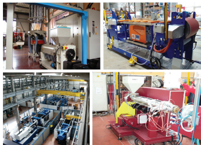
Examples of converting steps: (top): blown film extrusion, film take-off station, (bottom): injection molding facility, tube and profile extrusion machine (at IPC)
