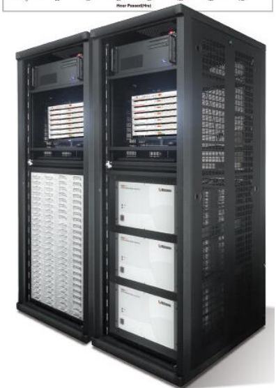
Testing OLED materials against continuous electrical source or environmental changes
