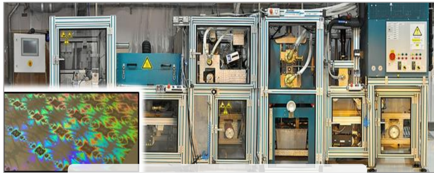
R2R micro- and nanostructuring
