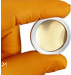
Case 2: gold coated polyester membrane for particle analysis of pharma liquids (case 2)
