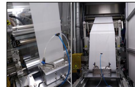
Coating of polymer film (left) and paper (right) at FhG-IVV.
