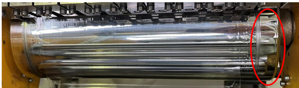
Figure 10. METEOR® PLA L175 on chill roll, liquid marked in red circle
